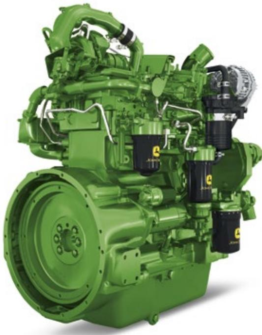
Our 4.5 l PSS engines (6110R, 6120R, 6130R and 6135R) use a 2-stage turbocharging system in which the VGT multiplies the pressure created by a fixed vane turbocharger. This sequential arrangement boosts power to achieve up to 166 hp (max with IPM) in the 6135R.
