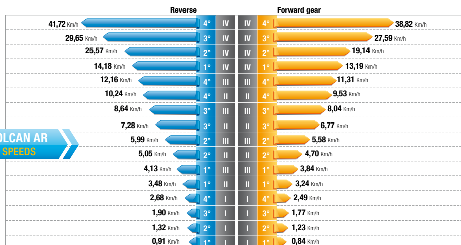
Graph of the speeds in km/h with 320/70R20 tyres for VOLCAN AR tractors. Engine speed: 2300 rpm
