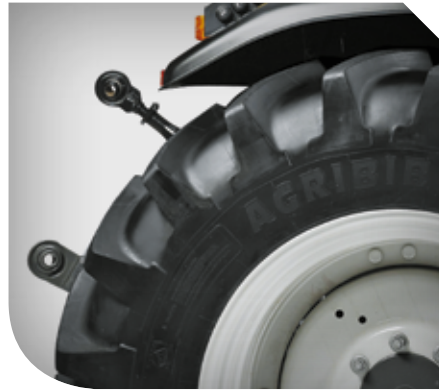
Linkage controls on the rear mudguard make working safe and practical. ( Standard in HiTech models, PTO controls as option ).
