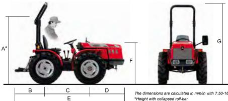
The dimensions are calculated in mm/in with 7.50-16 tyres \*Height with collapsed roll-bar
