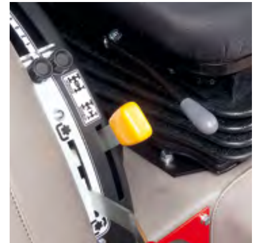
The front traction disengagement is useful when travelling along roads and prevents damage from being done to delicate grounds.
