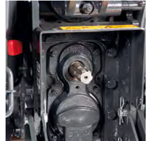
The PTO shaft of the ASAE 1 3/8 type is the same for all speeds.
