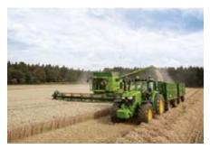
**On-the-go unloading** Thanks to John Deere Machine Sync the combine driver can adjust the tractor position to fully utilize the trailer capacity.
