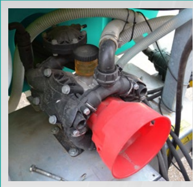
Membranska pumpa High pressure diaphragm pump
