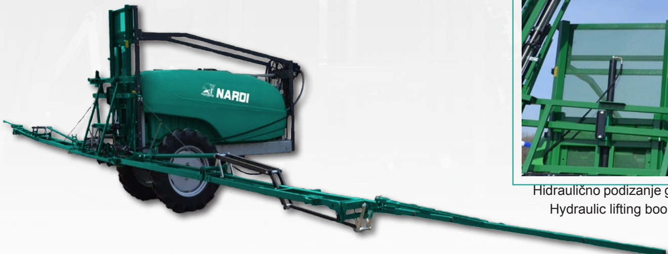
Hidraulično i mehaničko otvaranje grana Hydraulic & mechanic opening booms
