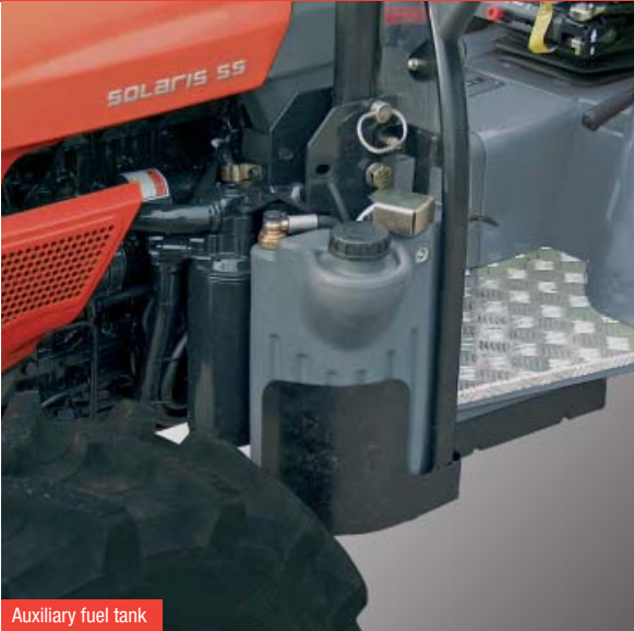
Auxiliary fuel tank
