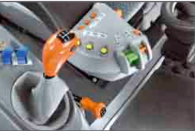
5-speed gearbox, 4 ranges (60 FWD + 60 REV), with creeper and H-M-L POWERSHIFT
