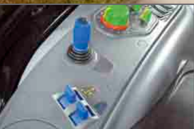
ENERGY SAVING electrohydraulic spool valves, 6/8 ports with flow regulator
