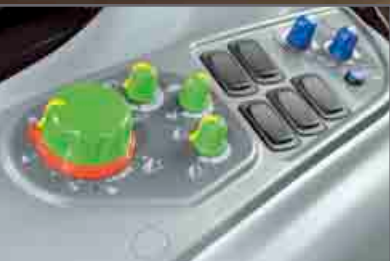
Electronic lift with maximum lifting capacity 6200 kg
