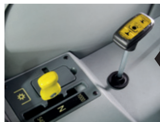
Selection of P.T.O. speeds is in the cab, on the right of the driving position.
