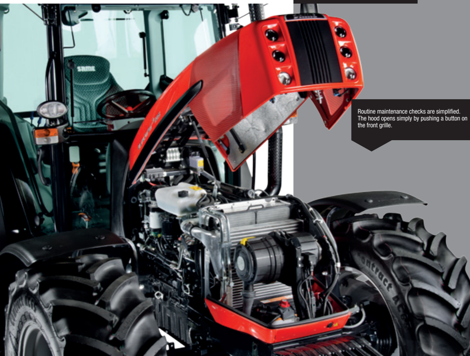
For maximum ease of maintenance, the radiator/cooler pack is equipped with a fly-screen that traps dust and other foreign matter.
