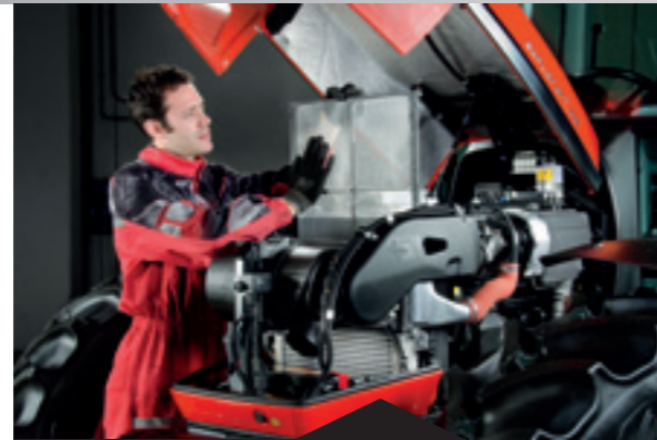
For maximum ease of maintenance, the radiator/cooler pack is equipped with a fly-screen that traps dust and other foreign matter.
