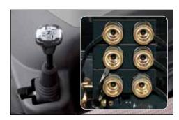
Remote hydraulic valve Standard dual remote hydraulic valves (3rd optional) accommodate a wide variety of attachments and implements. The Mid mount hydraulics and a single lever joystick for loader operations are standard on the RX series.
