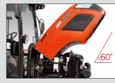
New elegant Grilland Hood New streamlined hood design improves visibility of the operator. The 60 degrees hood opening angle enables convenient access for better maintenance.
