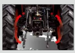
**External Hydraulic Cylinder** The RX series tractor has two external hydraulic lift cylinders(left and right) with highest lift capacity of 2,378 kg.f among its same class level tractors providing easiest condition for the maintenance.
