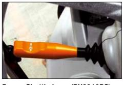
Power Shuttle Lever(RX6010PC) The Power Shuttle Lever provides easy forward and reverse operation without stepping on a clutch pedal.
