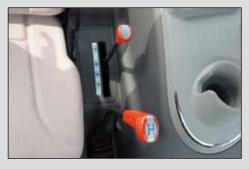
12×12 fully synchronized transmission The fully synchronized transmission provides smooth and easy shifting on the move. The transmission features 12 forward and 12 reverse condition. gears to handle all kinds of jobs.
