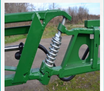
Sigurnosni zglob na kraju grane Safety joint at the end of the boom
