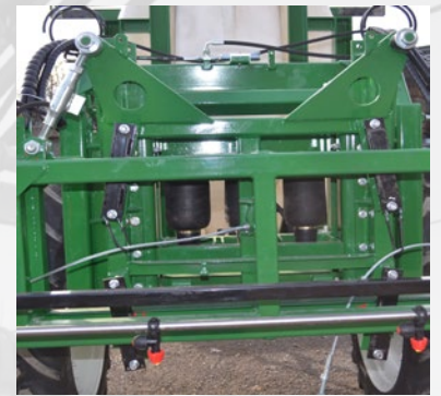
Vazдушna suspenzija grane Boom air suspension
