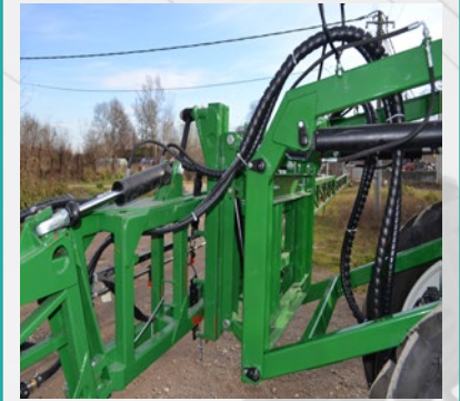
Hidraulično podizanje grana paralelogramom Hydraulic lifting booms with parallelogram
