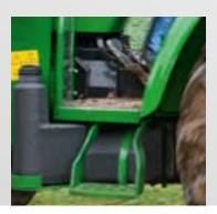
Optimised fuel tank The 68 litre fuel tank ensures easier access and better weight distribution
