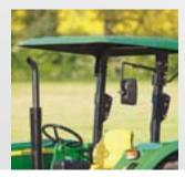
**Sun-protected**An optional roof provides you with protection from sun and precipitation
