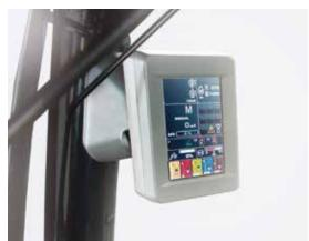
Everything is under control with the Nitro: the instrument panel boasts numerous indicators and warning lamps and a bright display, providing the driver with Information on vehicle speed, operating hours and distance in real time.
