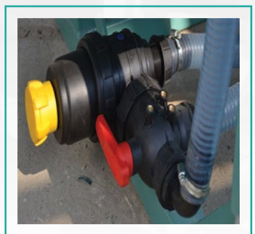
Filter za samopunjenje Intake filter predisposed for self-filling
