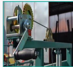
Čekrk za podizanje grana Winch lifting the booms
