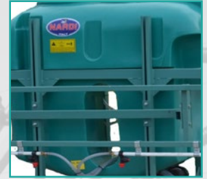
Ručno podizanje grana Manual lifting system of the boom
