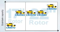
The performance of the CR combine is immediately obvious to customers. How? It's on the shielding. 'CR' stands for Rotary Combine. The first digit, either a 8 or a 9 refers to the size of the Twin Rotors. 8 for 17" models and 9 for the high capacity 22" variants. The final two digits, either 70, 80 or 90 indicate its position within the range. A higher number means a more powerful combine. Simple, isn't it!
