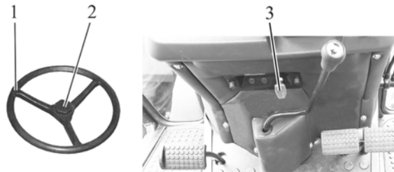
1 – steering wheel; 2 – chuck; 3 – handle to fix tilt of the steering column.
