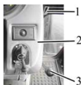
1 – instruction plate of fuel feed control; 2 – dashboard; 3 – handle of manual feed control.
