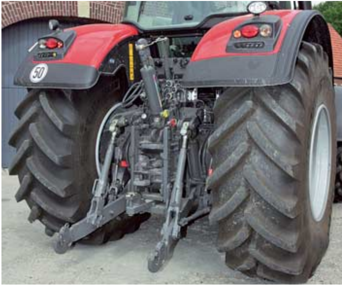
The MF 8690 linkage offers reasonable performance. Links on our test machine were category III. Photos: ST.
