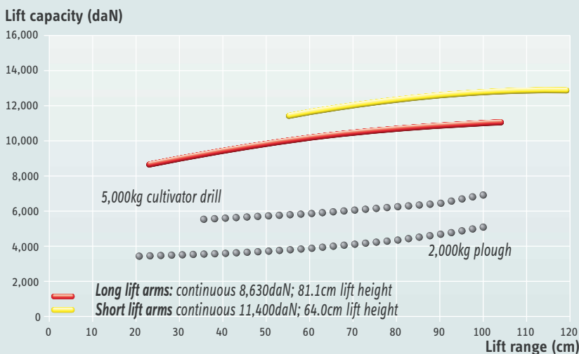
Massey Ferguson 8690: The red curve shows the recorded lift capacity (90% of maximum lift) as continuous lift power on the link ends. The yellow curve displays lift capacity with lift arms shortened – more than 2,770daN extra lift capacity, 17cm smaller lift range. Our MF test candidate boasted excellent lift forces.
