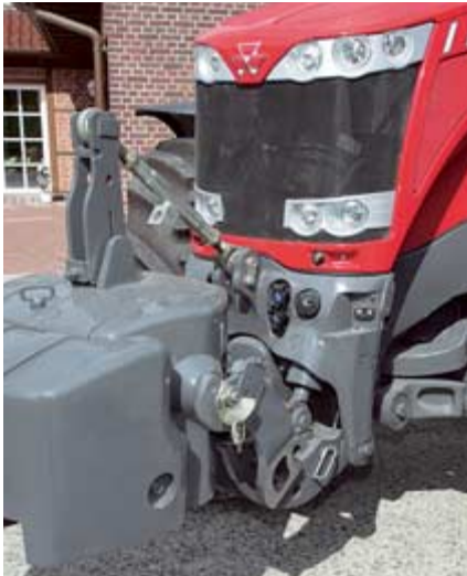
The MF 8690's integral front linkage is entirely new, and the operator can make the package double-acting by simply pressing on a button.
