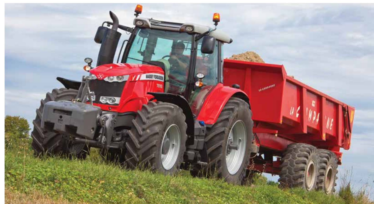
Dynamic Tractor Management (Dyna-TM) Intelligent machine management for optimum fuel efficiency Dyna-TM works in conjunction with Dyna-VT. This electronic management system automatically takes control of the engine and transmission when activated. Dyna-TM controls the engine speed according to the load on the tractor. It maintains the required forward speed whilst at the same time minimising the engine revs in order to keep fuel consumption to a minimum. Dyna-VT and Dyna-TM will work consistently at maximum efficiency and economy whilst maintaining a smoother drive quality and a noticeable reduction in fuel consumption.
