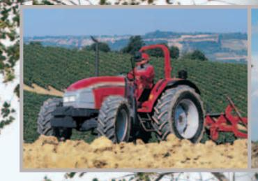
Designed by combining the features of two different tractor ranges, the new T-MAX (T3) inherits the cab and the wheelbase from the C-Max series and the 3-range Powershift transmission, the epicyclic final drives and the power lift from the new X60 series. The headlights and taillights, as well as the front grill, have been completely redesigned with a brand *new look*.
