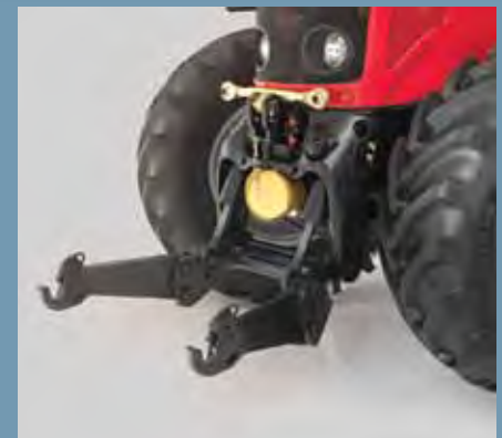
Massey Ferguson ILS features a fully integrated, factory-fit front linkage and PTO system.
