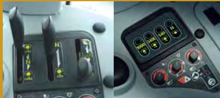
Convenient PTO speed selection (6400 Series shown on left, 7400 Series shown on right).
