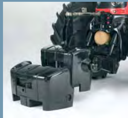
Front weight options, used with the ILS, include 1,323 lbs. (600 kg) and 1,984 lbs. (900 kg) modular front weights for balanced weight distribution.
