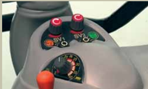
Control console for pedal/lever mode, High-Low (Rabbit-Turtle) range, SV1/SV2 cruise control setting and Engine Supervisor.
