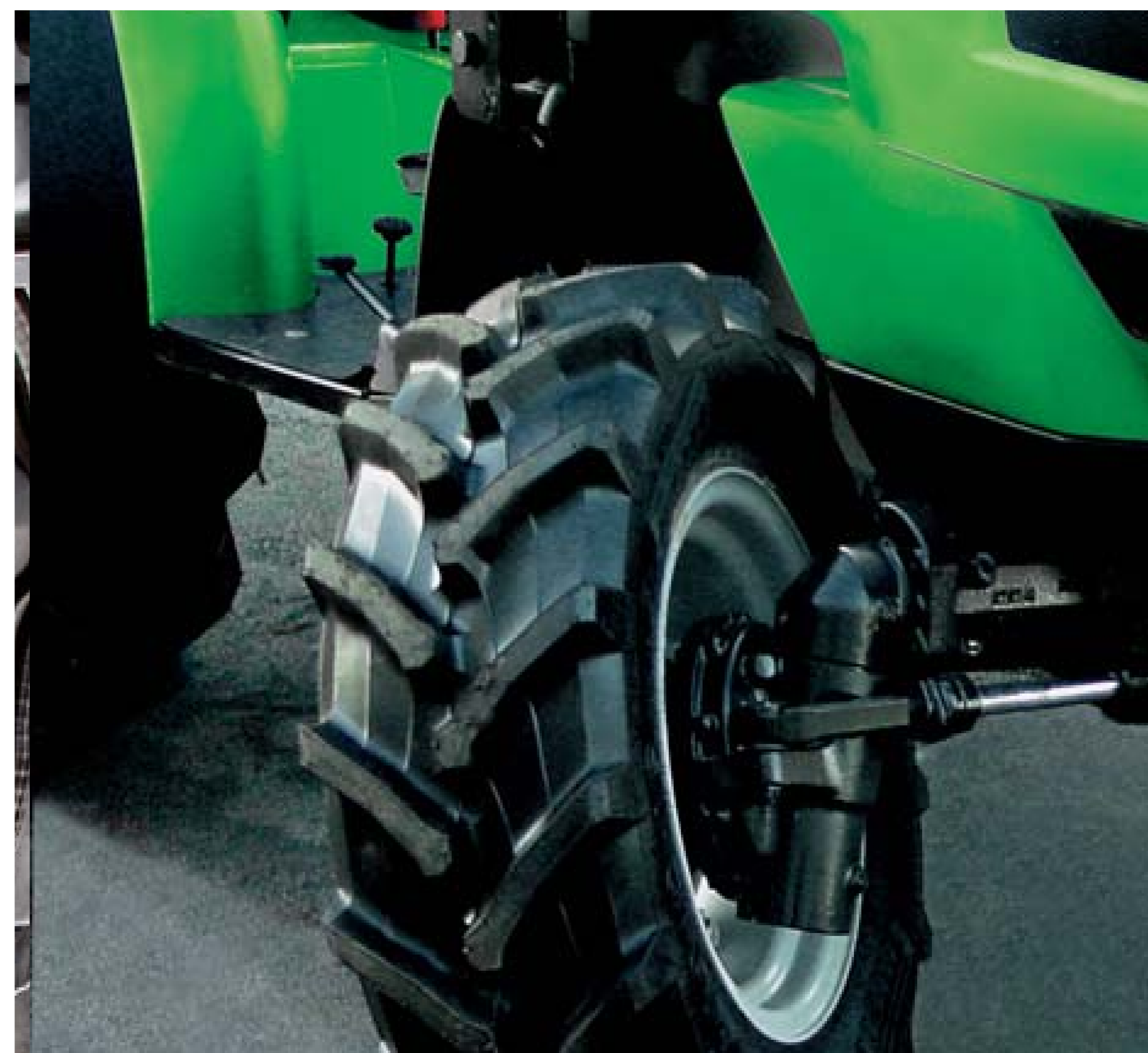
Tight, 102-inch (2.6 m) turning radius.
