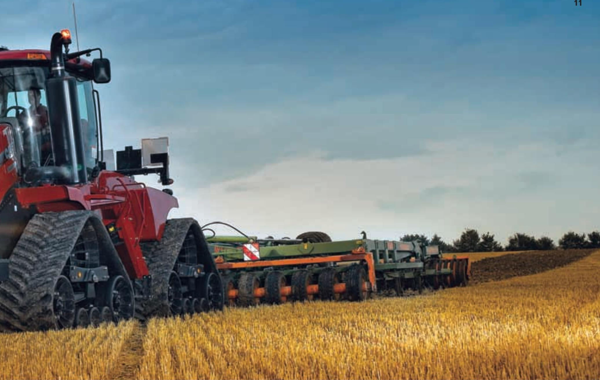
**Advanced Farming Systems** available on Steiger Quadtrac tractors are an essential ingredient for accuracy giving you improved efficiency. **ISOBUS implement interface**, a powerful connection to integrate and control ISOBUS compatible implements with the tractor AFS Pro colour touch screen monitor.
