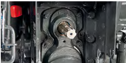
Two speed PTO: 540 rpm, 540 E (750 rpm) and synchronised with gear speeds. The PTO shaft of the ASAE 1 3/8 type is the same for all speeds.
