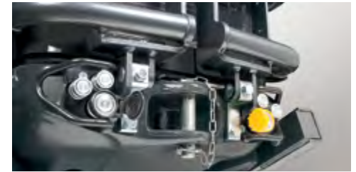
11 rear quick-couplers, 6 of which replicated at the front (opt).
