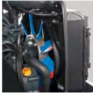
CLEAN FIX™ Reverse flow fan that assures the constant cleaning and efficiency of the radiator and of the front grille of the bonnet.
