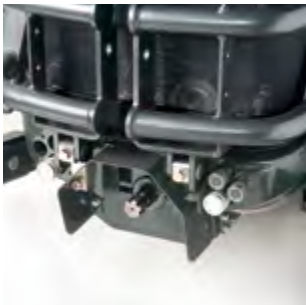
FRONT PTO The front PTO (1000 rpm) with electro-hydraulic controls and progressive engagement with safety button is maintenance free.
