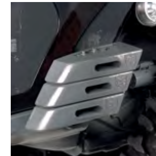
FRONT BALLAST Perfectly integrated into the bodywork of the tractor; it does not alter the wheelbase or dimensions of the tractor.
