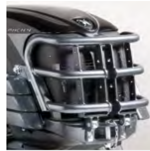
BULLBAR Tubular steel guard protecting the bodywork; integrates the third-point for the front lift.
