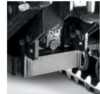
BALANCING BALLAST Supplementary ballast for optimising vehicle balance.
