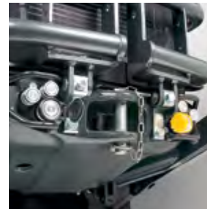
QUICK COUPLERS Front lift > 6 rear couplings.
