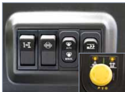
One touch PTO auto/manual and on/off switch, EHD and 4WD switch located in one place together.
