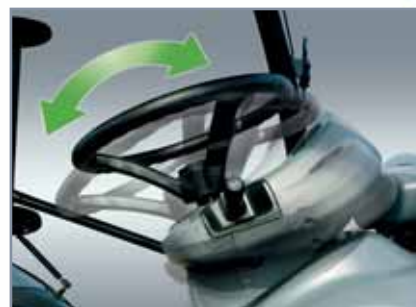
Integral steering wheel with tilting dashboard improve better visibility
