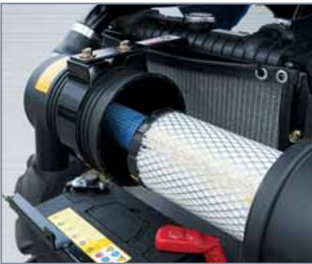
Dry air cleaner provides good accessibility and ensures longer engine life.
