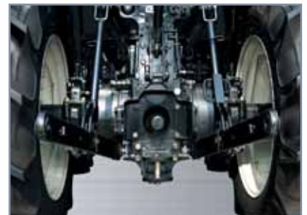
High PTO output and 3 PTO speed are standard (540/750/1000). (Option)
