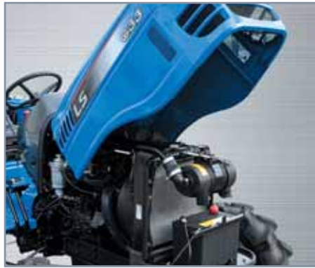
A customer-oriented bonnet allows convenient maintenance.
