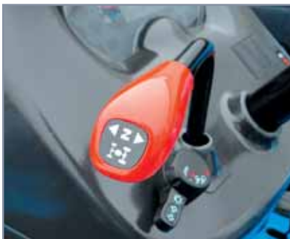
Synchromesh shuttle enables speedy operation.
