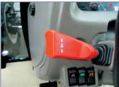
The superior finger-trip control type Shuttle Lever for forward/reverse shifting. (Option)
