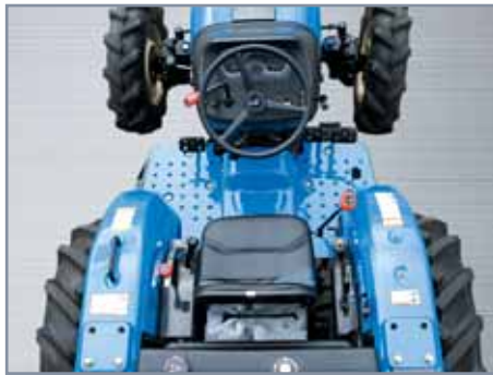
Semi flat deck gives operator more comfort when pushing down pedal and shifting gear lever.
