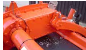
Intermediate drive for narrow transport width
