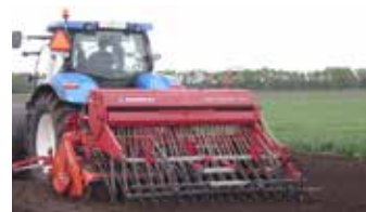
Combination with sowing machine and top-mounted lift
