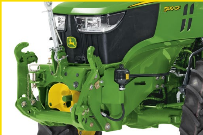
Both front and rear PTOs are offered with a choice of speeds.
