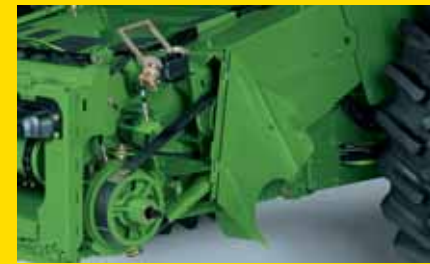
Feederhouse reverser – lets you remove the toughest clogs so you can get back to harvesting.
