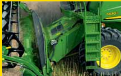
Adjustable feederhouse – maximises performance in all conditions from short, dry straw to long, wet crop.
