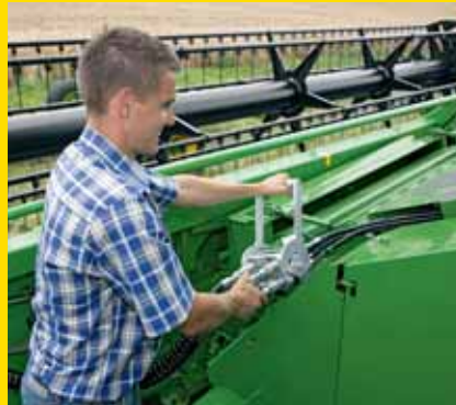
Single-lever multicoupler – provides the ultimate in header hook-up convenience.
