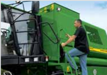
A pivoting ladder with four-step position offers easy access to the comfortable cab. Note the rails on either side of the ladder and the wide platform area. Excellent operator safety features are standard.
