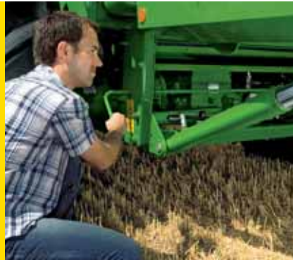
Stone trap – protects the cylinder and concave. Open and empty with just one lever.
