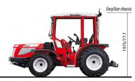
The dimensions are calculated in mm/in with 260/70 R16 front, 300/70 R20 rear tyres \*Height calculated with the operator of average height sitting (mm/in 1750/68.9)
