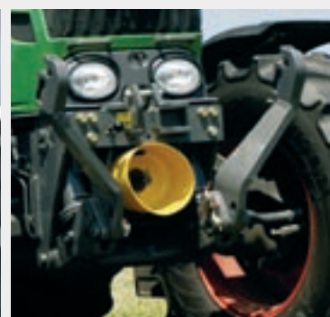
Integral front power lift and front PTO
