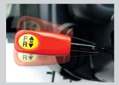
**Power ShuttleTransmission** The 16X16 Power Shuttle Transmission comes standard with Kioti's DX series tractors. This transmission provides easy forward and reverse operation without depressing the clutch pedal. This feature also reduces the opreator's fatigue dramatically and is perfect for loader works.
