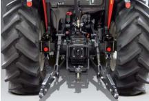
**Telescopic CAT II Hitch** Category II 3-point hitch with standard telescopic link ends make attaching implements quicker and easier than fixed links and enhances operator's safety. The DX series come standard with telescopic stabilizers and a RH leveling box to provide operator's with a wide ranges of customizable 3-point hitch options depending on the job at hand.
