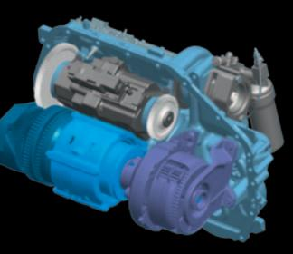
without the classic "jolts" noticeable when changing gear using traditional transmissions. The two elements of the continously variable transmission are connected to a geared control unit. The assembly is completed with an electrohydraulic shuttle and controlled by an advanced electronic control unit (ECU) that continuously "talks to" the engine control unit to seek maximum efficiency for each operating condition.
