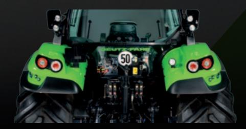
The Power-Beyond hydraulic coupler allows full oil flow from the pump to be distributed to one or more hydraulic motors on an attached implement. This is an extremely useful feature when using implements that have their own hydraulic power drive. The high capacity improves hydraulic system performance and helps keep down fuel consumption.
