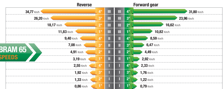
Graph of the speeds in km/h with 33x15.50-15 tyres for COBRAM MT tractors.
