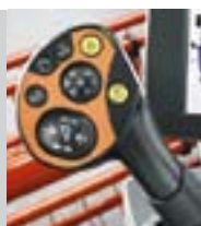
The automatic cutterbar control is activated simply by pressing the button for height adjustment on the multifunction control lever.
