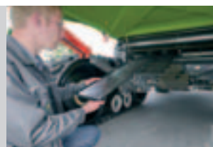
Divided grain pan that can be removed from the front
