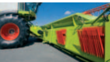
Additional crop lifters stored directly on the cutterbar
