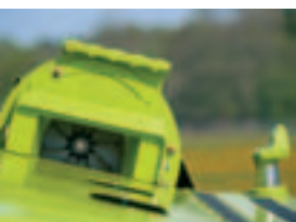
For a clear view: dust extraction at the feeder housing
