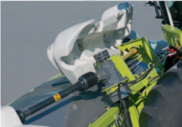
Paddle roller height is adjusted hydraulically
