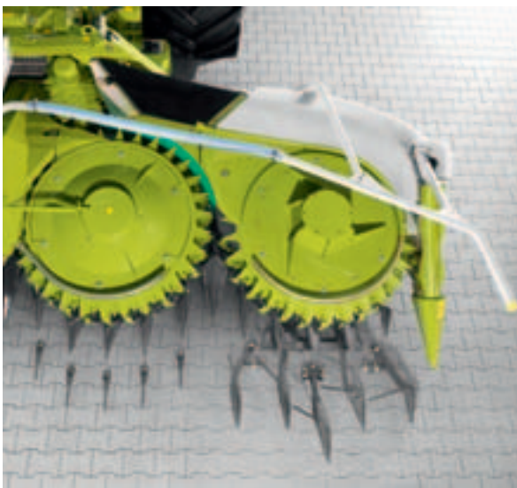
Finger extensions, attachable points and feeding drums for different operating conditions
