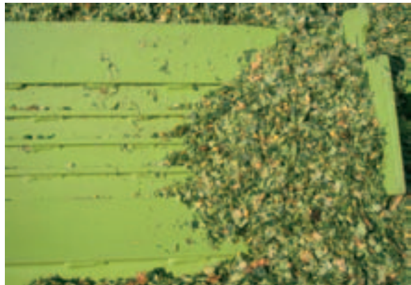
The friction concave plate: it can be fitted under the knife drum as an alternative method of processing the chopped material
