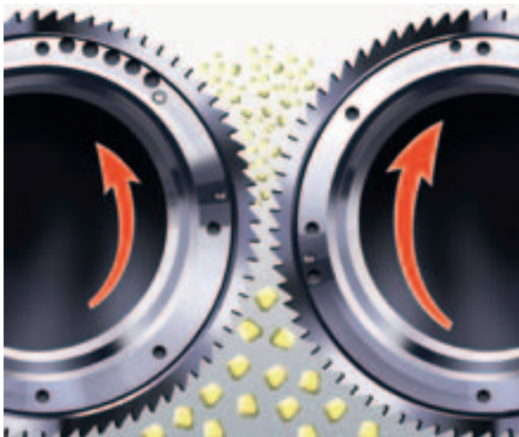
Functional principle of a high-performance cracker with saw-tooth profile
