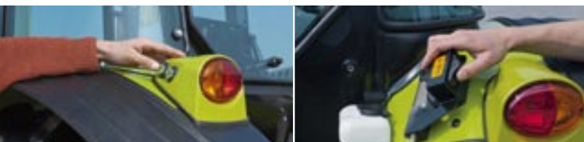
Convenient external control with mechanical or electronic rear linkage.
