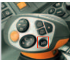
Guidance system activation button on CMOTION
