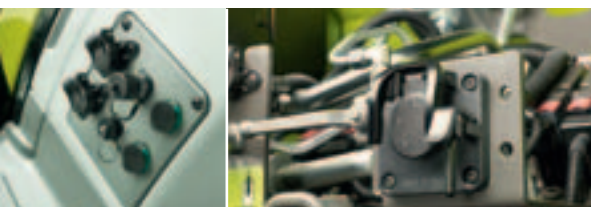
ISOBUS connectors in the cab and at the front and rear.
