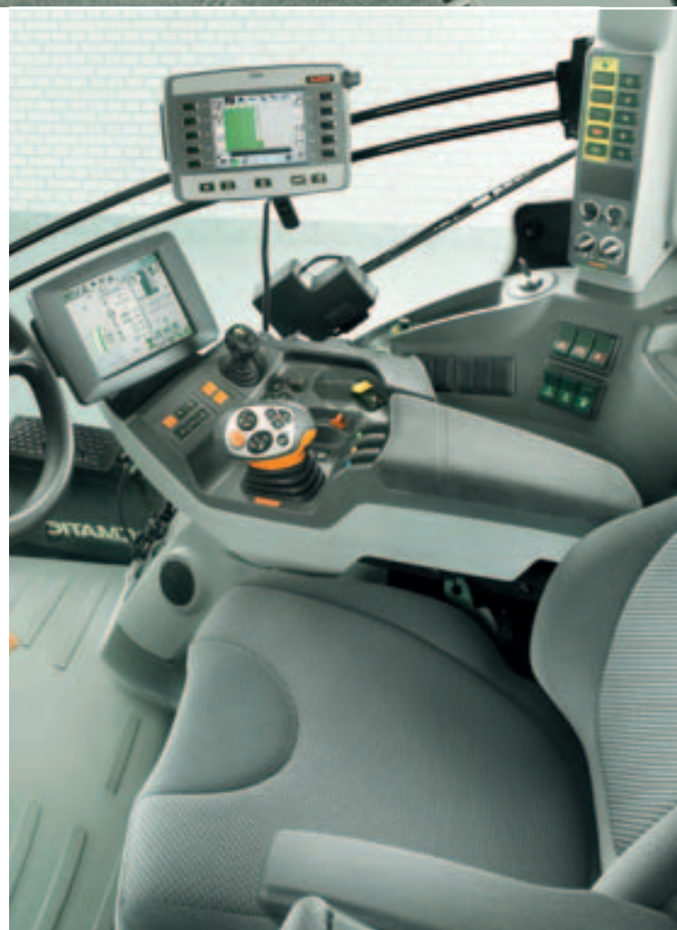
Control panel (11) in the armrest: four-wheel drive, differential lock, automatic PTO engagement/disengagement and front axle suspension
