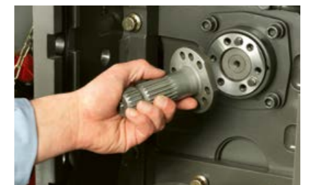
The PTO stub can be changed easily
