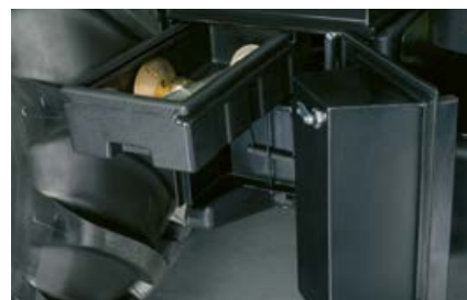
The battery and a tool storage compartment are handily located in the access ladder on the right-hand side.
