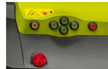
External controls for rear PTO
