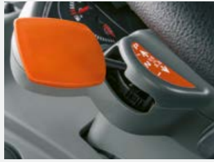
NEW: REVERSHIFT shuttle lever with electronic parking brake available
