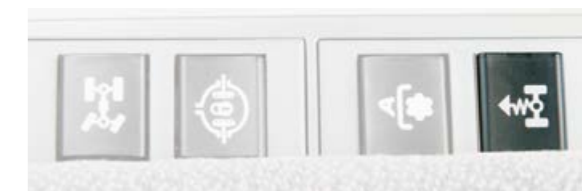
Switch to activate front axle suspension
