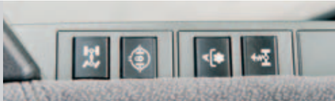
Control panel (11) in the armrest: four-wheel drive, differential lock, automatic PTO engagement/disengagement and front axle suspension
