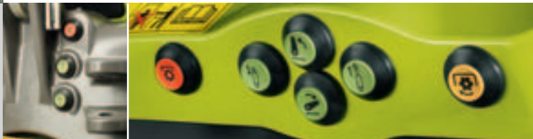
External controls for front and rear PTO
