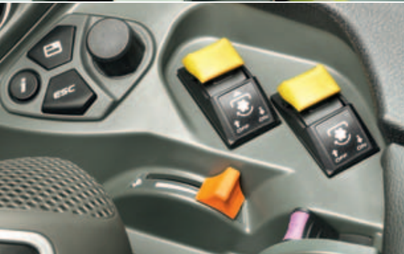
External controls for front and rear PTO
