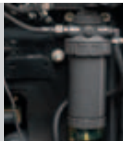
The fuel prefilter is conveniently located by the steps to the cab.
