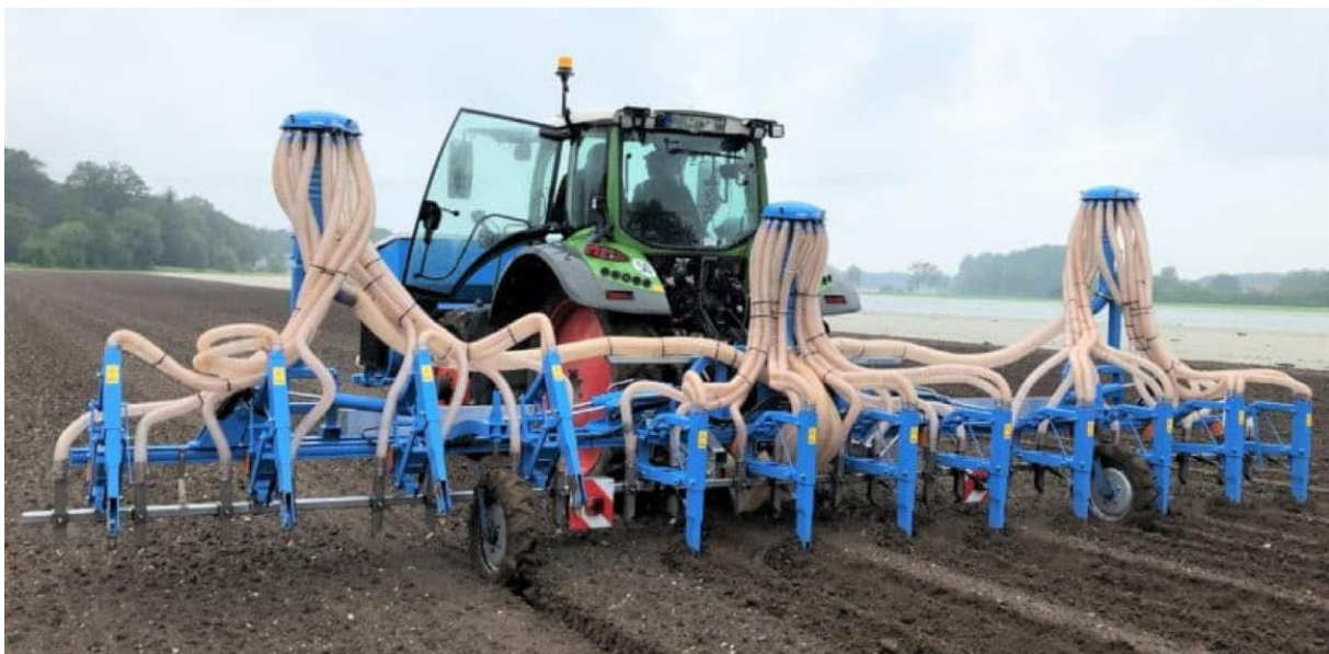
Figure 2: Subsurface fertiliser application – one option to improve nitrogen use efficiency.
