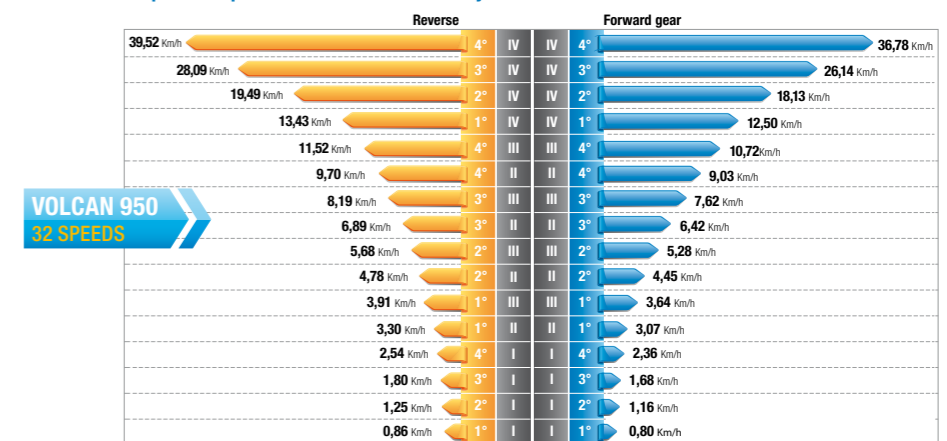
Graph of the speeds in km/h with 340/65R20 tyres for VOLCAN MT tractors.
