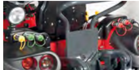
Hydraulic system with 4 double-acting manifolds, 1 single-acting, 1 continuous flow manifold + oil return tap.
