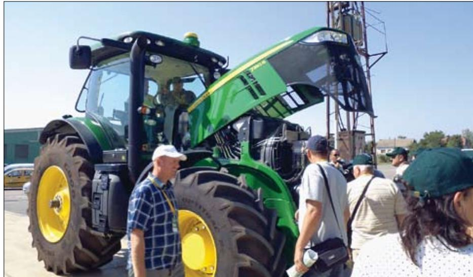
John Deere 9,0 L PowerTech Plus motor na 7280 R
