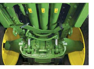
A | Transmission Output Shaft B | Double Reduction Front Axle C | Front Suspension Cylinder
