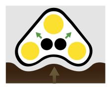
**9RX design:** The innovative 2 mid-roller design of the 9RX helps dissipate vibration, diverting it away from the axle and ensuring a safer, more comfortable ride.
