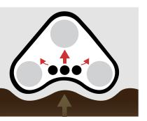
Alternative design: With 3 mid-rollers, vibration is transferred directly upwards into the drive sprocket and axle. This makes for an uncomfortable ride.
