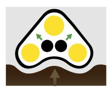
**9RX design:** The innovative 2 mid-roller design of the 9RX helps dissipate vibration, diverting it away from the axle and ensuring a safer, more comfortable ride.
